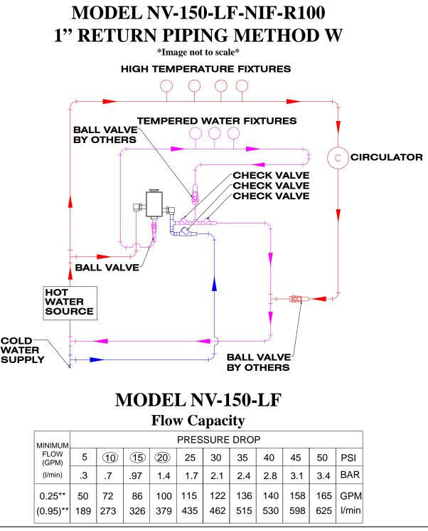
NOTE: Flowrates will vary depending on existing field conditions. Leonard Valve Company always recommends using CASPAK® sizing software for proper valve sizing and model number applications.
